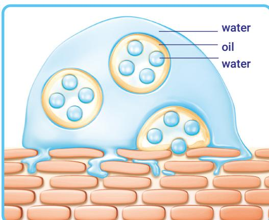
Multi-phase water-in-oil-in-water system
